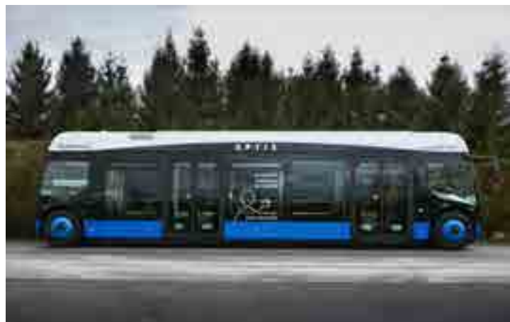
Aptis (above) is a rubber-tyred bus/tram hybrid. The Coradia iLint (above right) is powered by hydrogen from an industrial process
