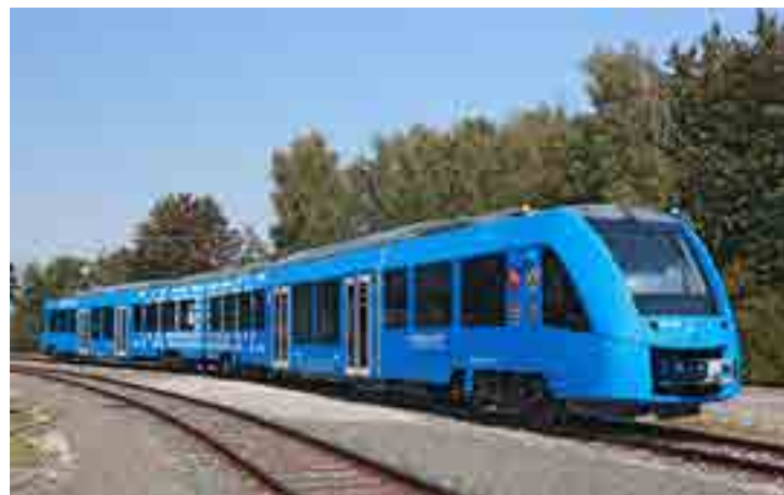
Aptis (above) is a rubber-tyred bus/tram hybrid. The Coradia iLint (above right) is powered by hydrogen from an industrial process
