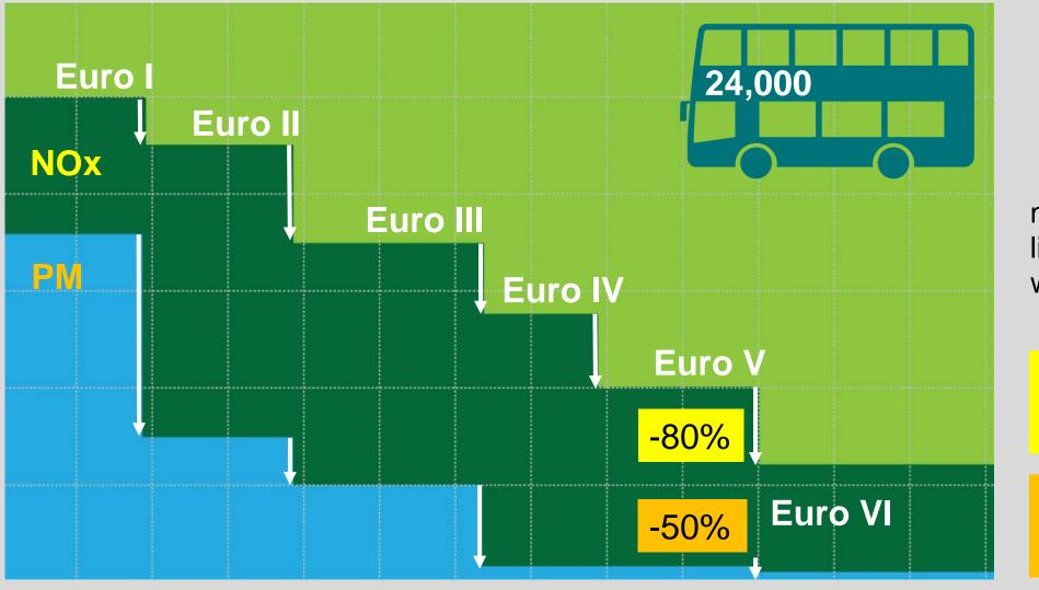
mass emissions limit per unit of work in kilowatt-hours
